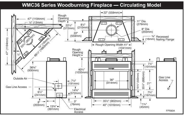
Fig. 1 WMC36 Series specifications and framing.
